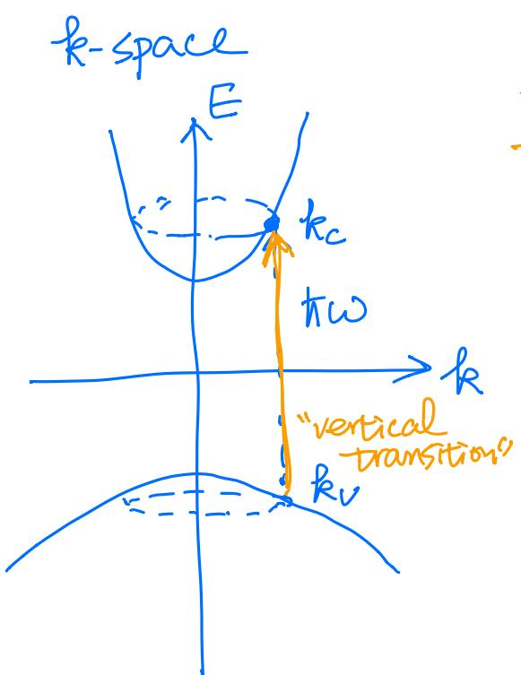
$$R_{V \rightarrow C} = \frac{2}{V} \sum_{\vec{k}_c = \vec{k}_v} \frac{2\pi}{h} |H'_{cv}|^2 \delta(E_e - E_h - \hbar\omega) f_v (1 - f_c)$$
